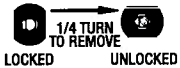
LOCKED UNLOCKED IMPRESSION "A" IS REMOVABLE WHEN USED WITH A D-SHAPED STUD
